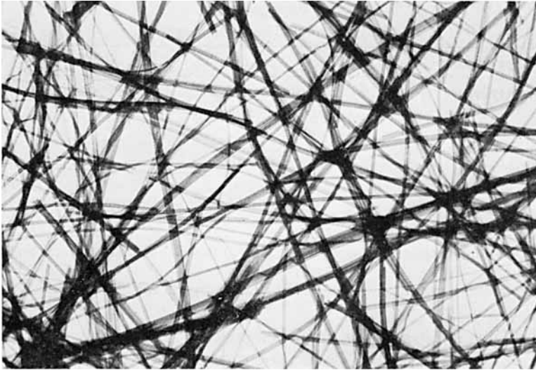
Fig. 1. Electron micrograph of chrysotile asbestos (Plastibest No. 20) dispersed with sodium polyacrylate. 10,450 \times .
