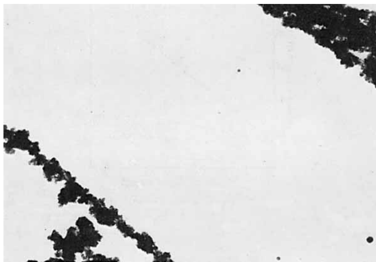
Fig. 9. Electron micrograph showing completely coated chrysotile fibers. Copolymerization of styrene 1 DMAEMA (3/1) in the presence of PAA (AIBN as initiator). 5,010 \times .
