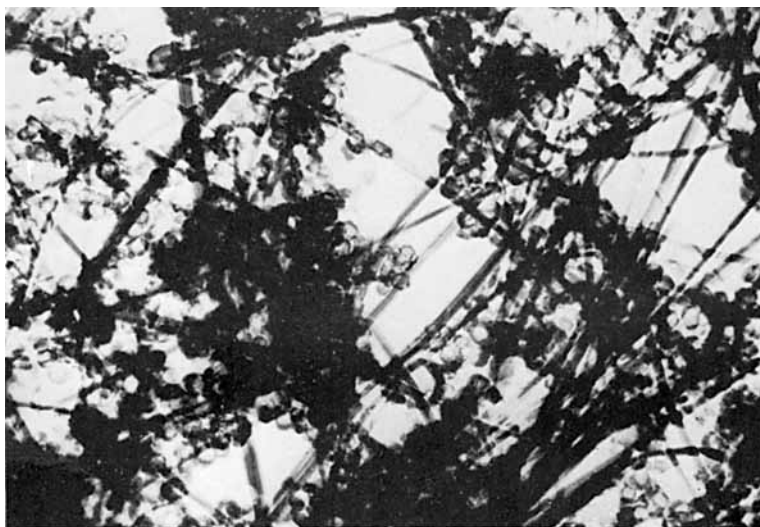
Fig. 5. Poly(methyl methacrylate) particles formed in the presence of asbestos dispersed with sodium polyacrylate ( K_2S_2O_8 as initiator). 16,500 \times .
